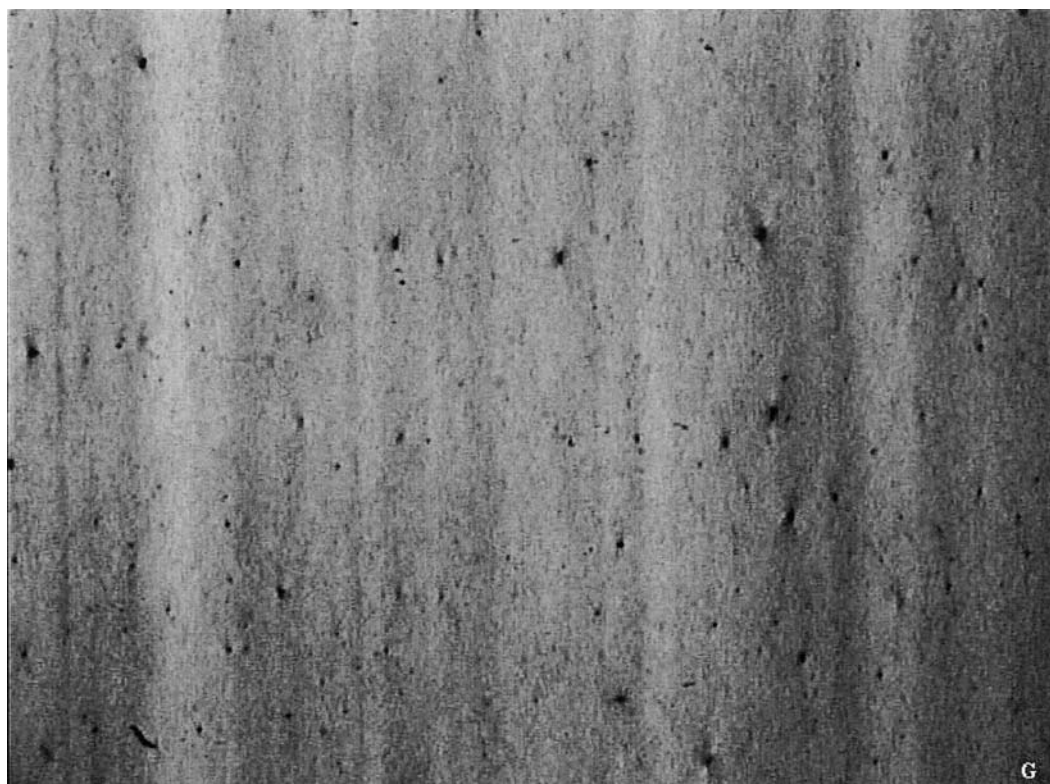
FIG. 13—Low-density bags: pattern of extrusion lines (over a few centimeters), visualized by means of transmitted light.
