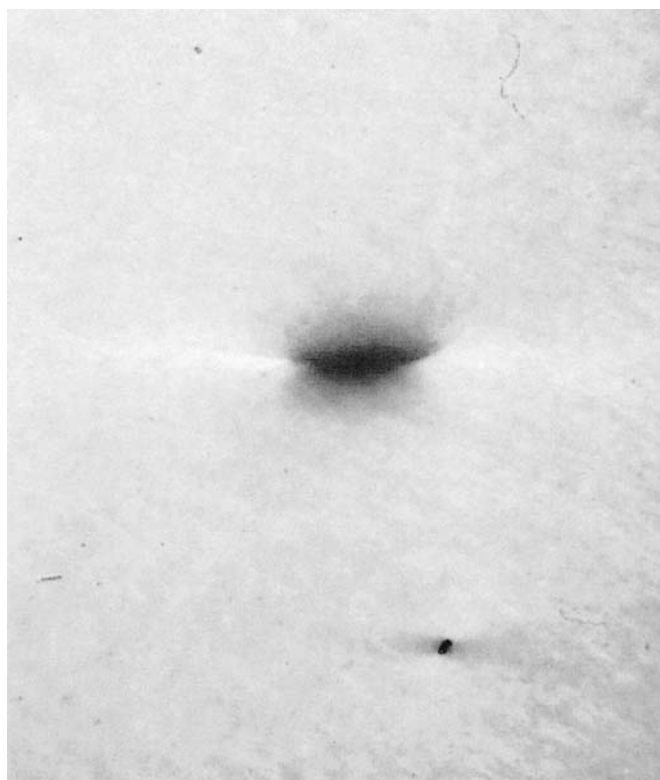
FIG. 2—Visualization by means of transmitted light of two so-called “fisheyes,” dark scattered spots with light-colored tails.
